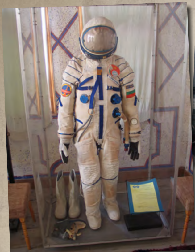
The "Sokol" space suit, developed by the Space Research Institute at the Bulgarian Academy of Sciences and used by the cosmonauts Georgi Ivanov and Alexander Alexandrov
